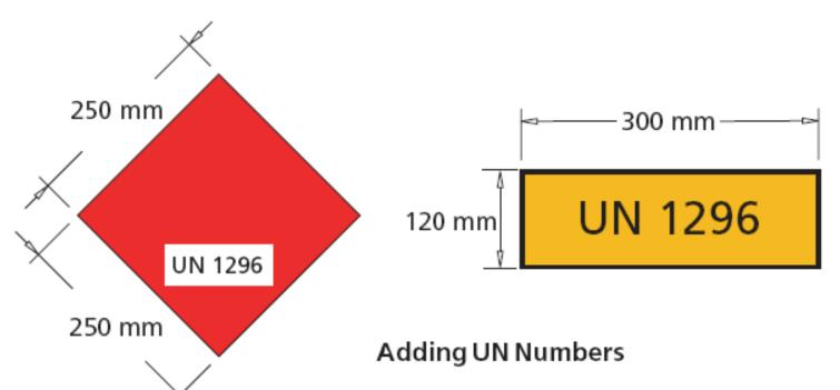
Two acceptable ways of adding UN numbers to placards on cargo transport units.
