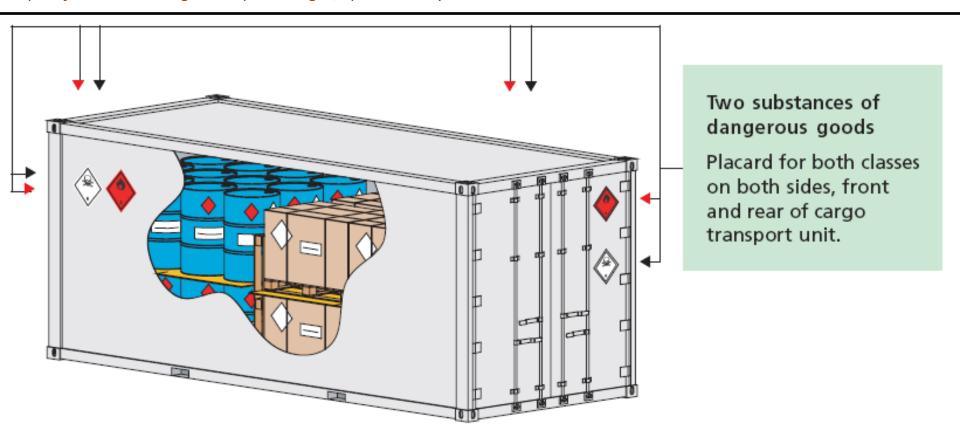
Above: IMDG Placard requirement for two dangerous substances, both with a single hazard class.
